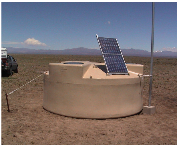
Fig. 1. 12,000 liter Polyethylene rotomolded tank for the Auger ground array
