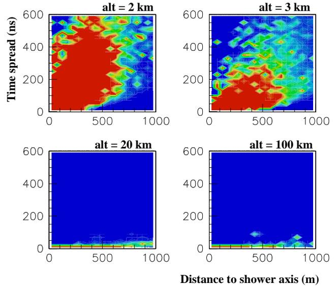
**Fig. 2.** Particle time spread with respect to a planar shower front versus distance to the shower axis for  $10^{19} \text{ eV}$  protons at 80 deg zenith angle. The primary altitude is given at the interaction point, early interactions (bottom) correspond to high altitude and produce old shower at the ground level, late interactions (top) correspond to penetrating particle and young shower.
